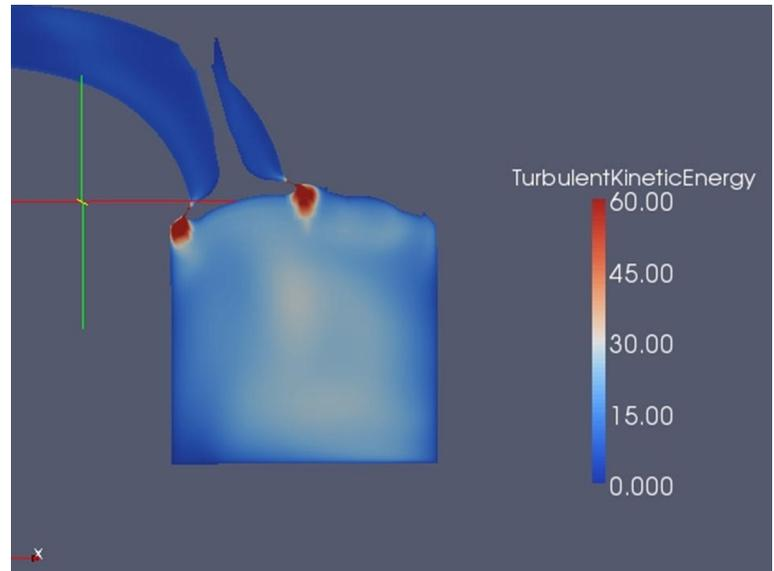
Varying the piston stroke causes variations in internal turbulence with negative consequences on engine thermal efficiency
