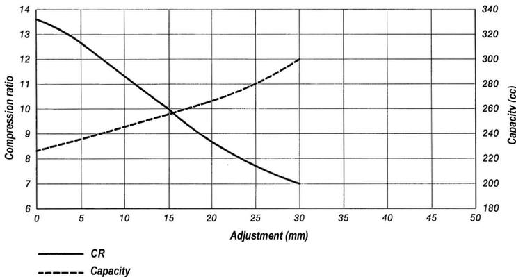
Various VCR concepts and applications exist that aim to make compression ratio and capacity vary simultaneously
