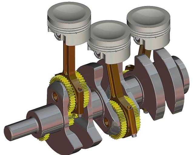
The GoMecsys concept enables the differentiation of the intake-compression stroke from the expansion-exhaust stroke
